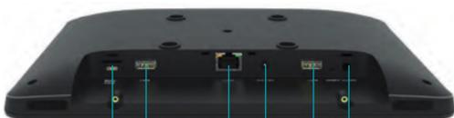
Micro SD    USB    Ethernet    DC in    USB    Audio Out
